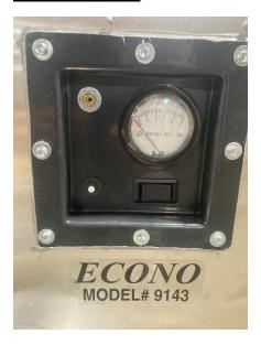
Contains helic gauge, LOW/HIGH OFF switch and circuit breaker
